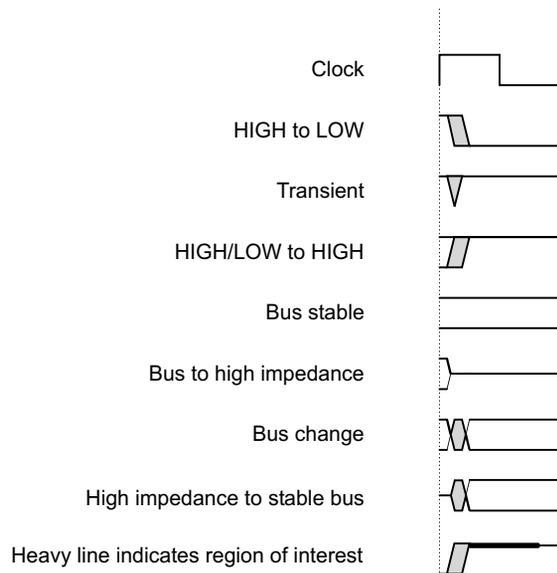
**Figure Pre-1 Key to timing diagram conventions**
