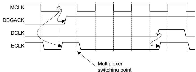
Figure 5-4 Clock switching on entry to debug state
