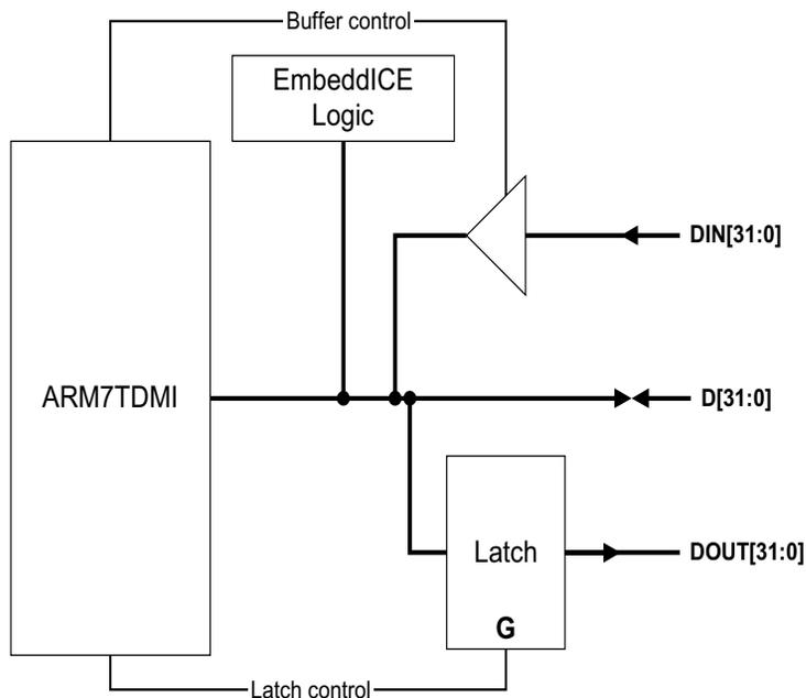
**Figure 3-11 External bus arrangement**
