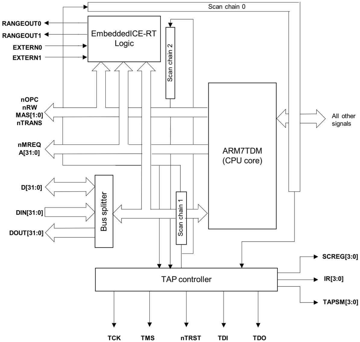
Figure 1-2 ARM7TDMI processor block diagram
