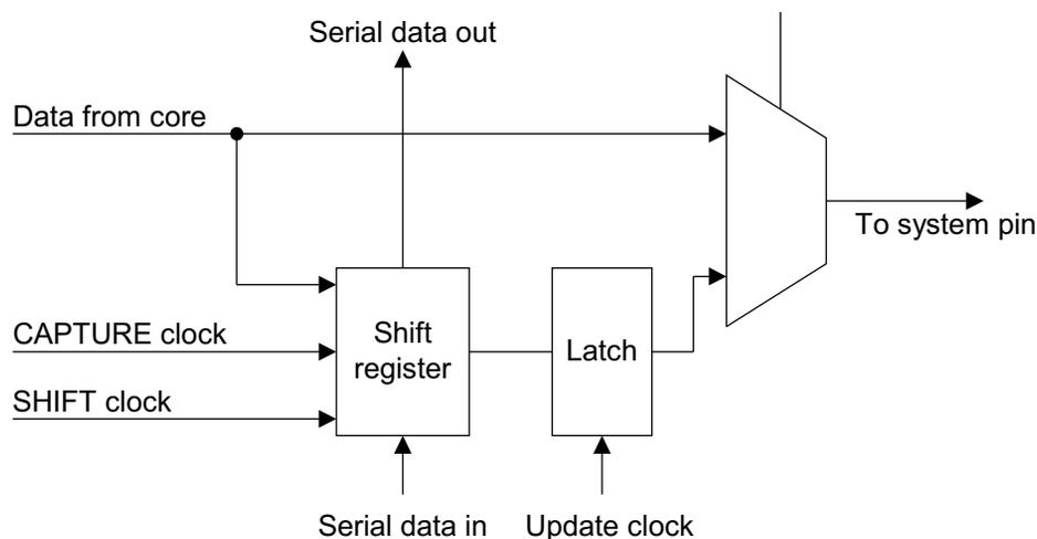
**Figure B-4 Output scan cell**
