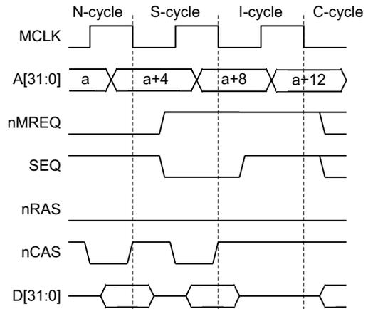
**Figure 3-4 Internal cycles**
