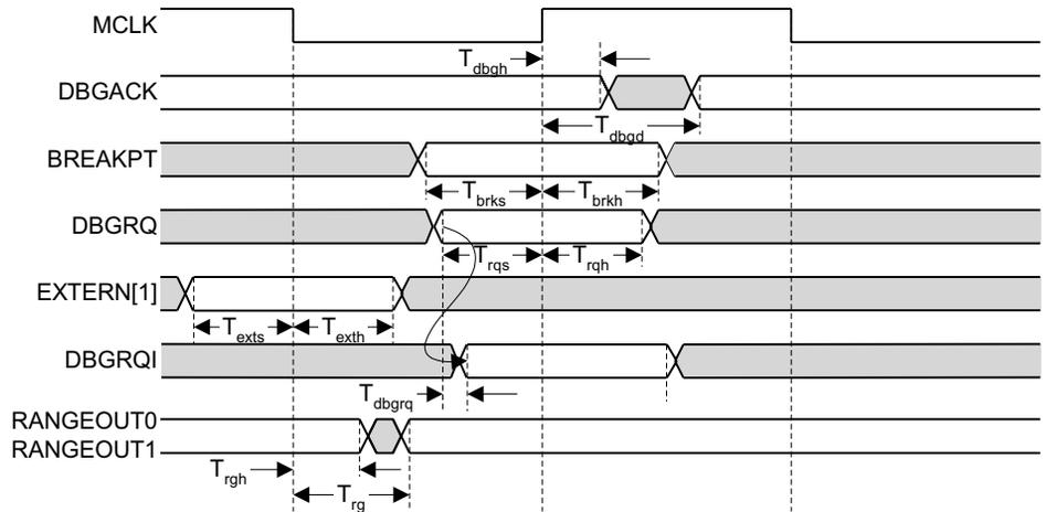
Figure 7-13 Debug timing
