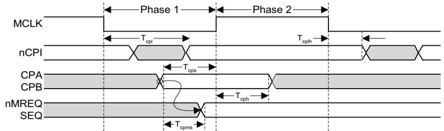
Figure 7-10 Coprocessor timing
