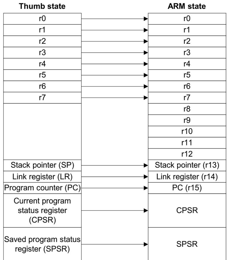
Figure 2-5 Mapping of Thumb-state registers onto ARM-state registers
