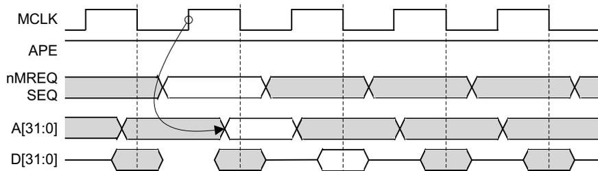
**Figure 3-8 Pipelined addresses**
