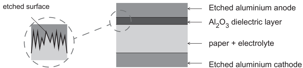
Figure 3.13 Electrolytic capacitor construction
