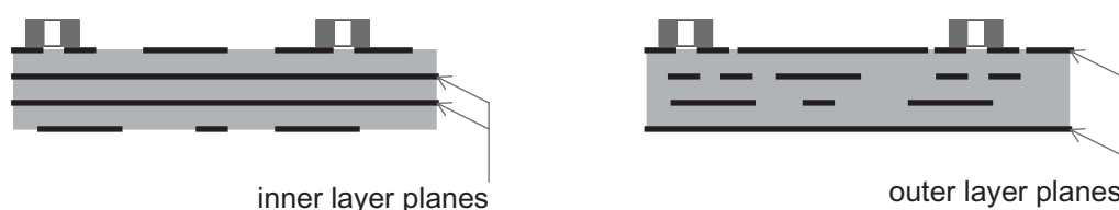
Figure 2.9 Inner layer vs. outer layer planes
