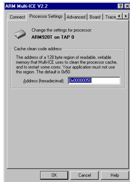
Figure 4-11 Multi-ICE Processor Settings tab showing cache setting
